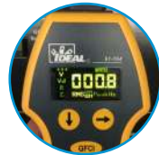
Displays neutral to ground voltage
