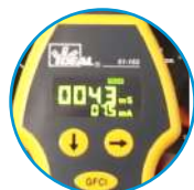
Trips GFCI at 6mA or 30mA
