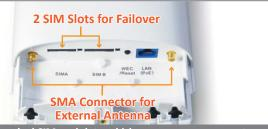
AirMax4GW has dual-SIM card slots, which means you can connect selectively to two carrier networks. When the network over the primary SIM fails, the AirMax4GW will automatically switch to the secondary SIM card and continue working without any latency.
