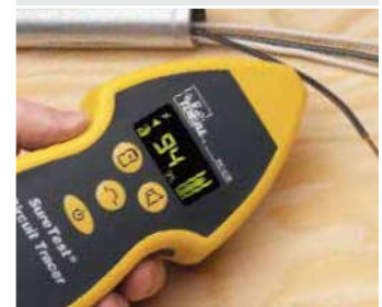
Individual wires can be sorted, opens can be located and shorts can be isolated.
