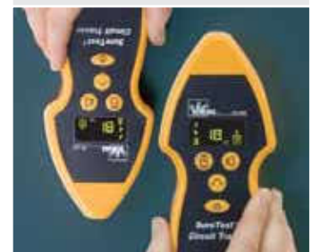
Display rotates in 90° increments so that you always receive an upright reading.
