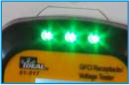
Green Lights Indicate Correct Wiring
