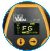
Detects and Displays false or "bootleg" ground
