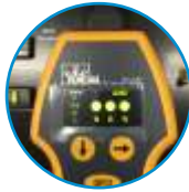
Displays H N G polarity
