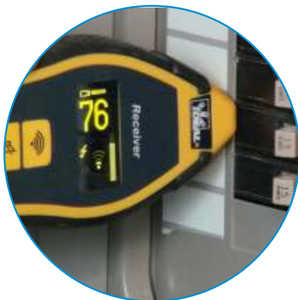
Finding Breakers or Fuses
