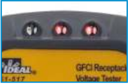
Red Lights Indicate Incorrect Wiring
