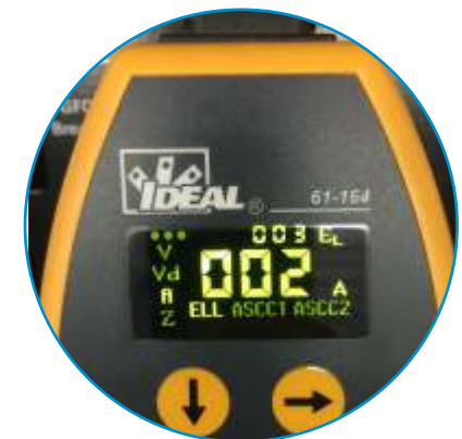
Estimated Load on Line in Amps
