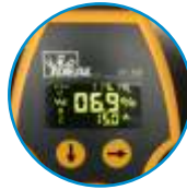
Displays Voltage Drop at 12, 15 & 20 Amps
