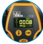
Displays neutral to ground voltage
